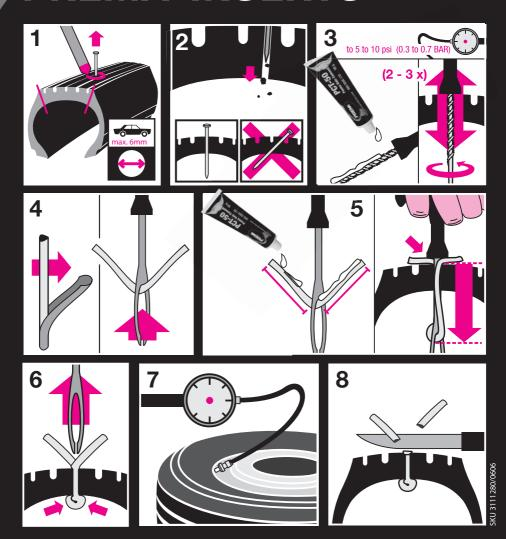
WARNING: The PremaFill product is intended for temporary use only until the tire can be removed from the rim, inspected, and permanently repaired in accordance with industry standards. Permanent repairs can be performed using a Prema Combi Unit, Prema Universal Repair/Prema Stem combination, or Prema Reinforced Repair/Prema Stem combination in accordance with the appropriate Prema Nailhole Repair Manuals.
